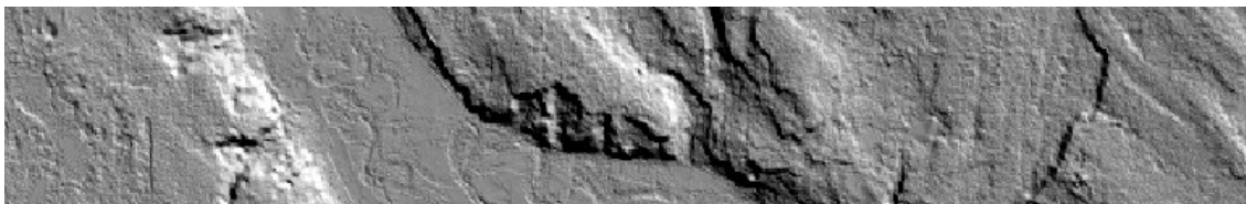
Fig 3 InSAR Derived DTM. Sample size: 2x10km (after Norheim et al, 2002)
